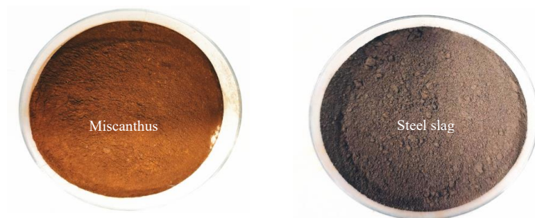
Fig. 5.1 Heat-treated miscanthus powder and steel slag powder and their microscopic images.
