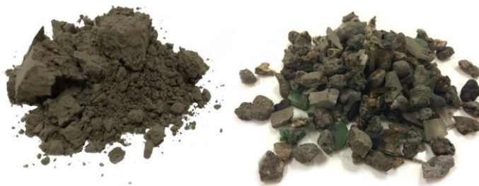
Figure 1.3 MSWI bottom ash used in the study: fine fraction (< 63 \mu\text{m} ) (left) and large fraction (22.4 mm) (right) (Mineralz, the Netherlands).
