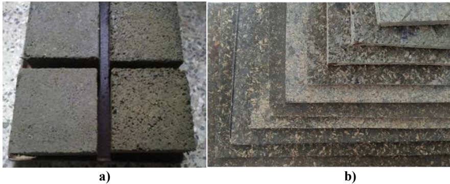
Figure 2.1: Illustration of cement-fibre composite: a) lightweight concrete (wood fibres waste, rice husk ash) [57]; b) cement-bonded composite (a combination of different chemical additives and press time) [58]
