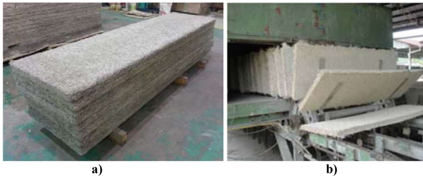
Figure 2.2: Illustration of cement-fibre composites – wood-wool cement boards: a) wood-wool cement boards; b) curing process of WWCB [59]
