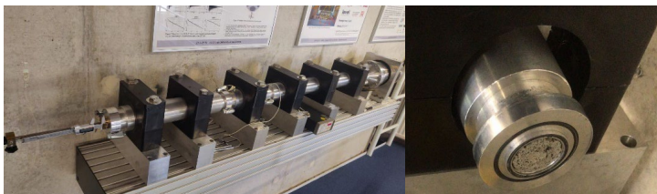
Fig. 2.1. Measurement of acoustic absorption of porous composites.
