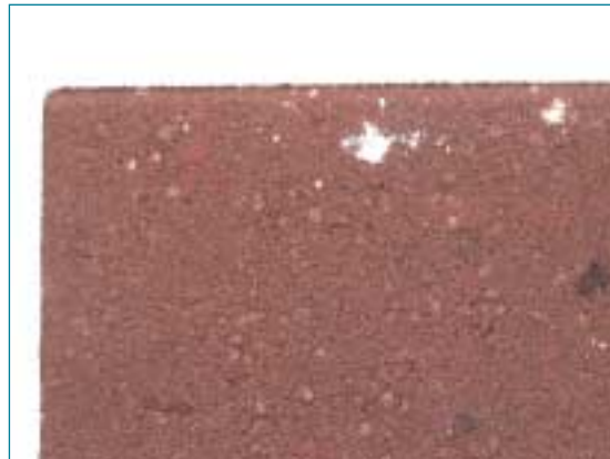
Fig. 2 Agglomerates of TiO 2 formed at the surface of a concrete paving block.
