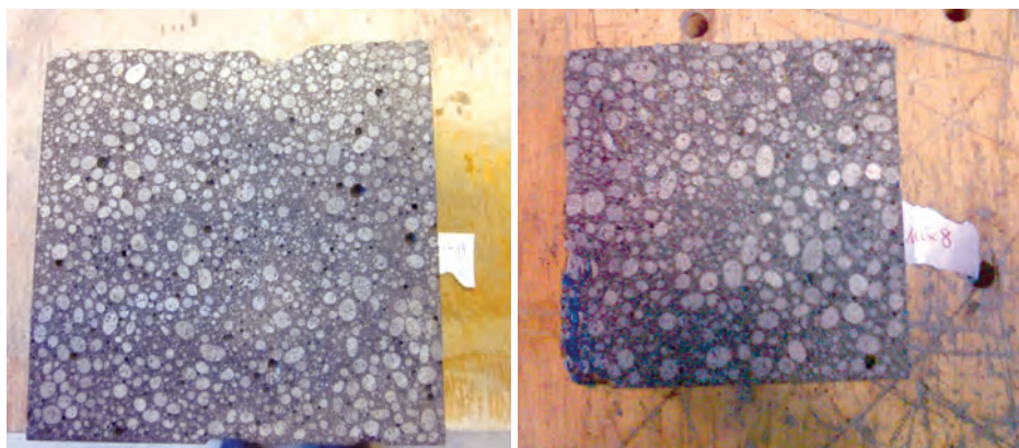
Fig. 2. The pictures of a cut surface of LWAC from two mixes
