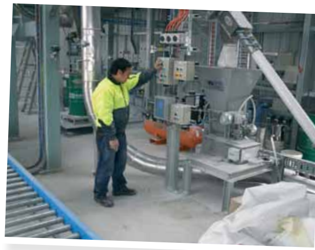
Figure 2. Calix CFC plant showing the continuous feed of ground magnesite into the steam flow for injection into the CFC Calciner.
