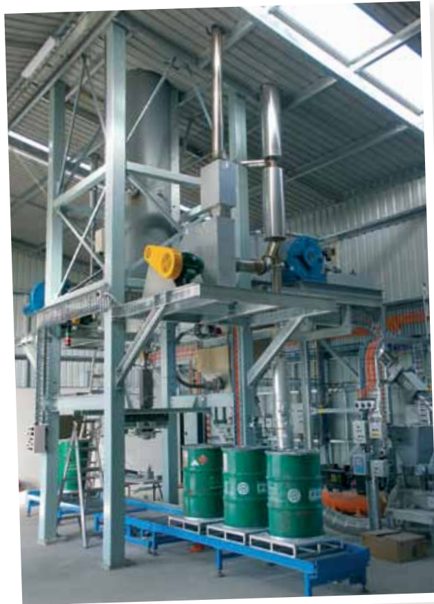
Figure 1. Calix CFC plant at Bacchus Marsh Victoria showing the production of drums of calcined magnesite from the 12 m CFC Calciner seen in the upper left.
