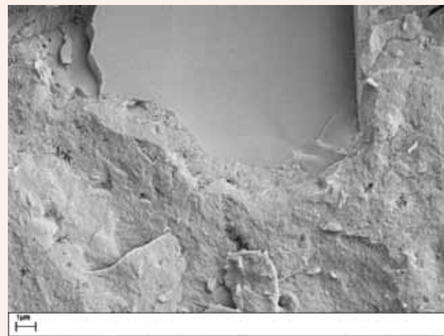
Figure 2. Cryo-REM image of a broken Celitement paste after 7 days' hydration. A silica-rich core is enclosed in hydrated calcium silicate hydrate. Pore space is nearly closed. Image width 22 \mu\text{m} .
