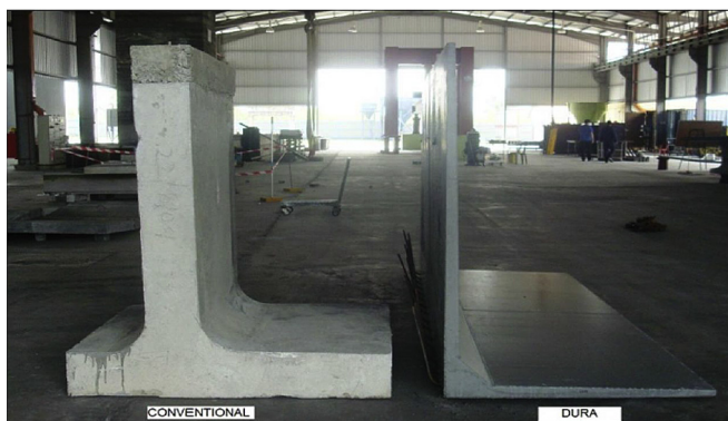
Fig. 1. Difference in sectional dimensions of an L-shaped wall, made of conventional concrete and UHPFRC (Voo et al., 2012).
