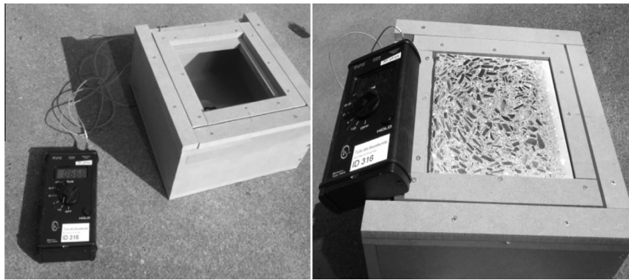
Fig. 3. Translucency measurement test set-up.
