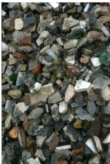
Fig. 2. Bottom ash granulate fraction 8–16 mm.
