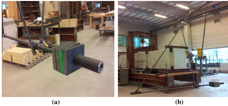
Fig. 8. Constructed hammer, (a) hammer head; and (b) hammer arm in the set-up.
