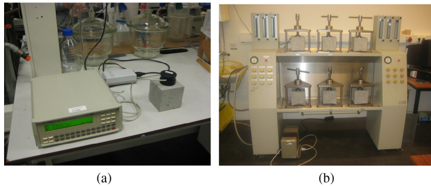
Fig. 3. Test pictures of (a) thermal property; (b) water penetration under pressure.
