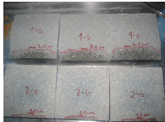
Fig. 17. Split surfaces of cubes after the water pressure permeability test; water ingress from the side of the bottom surface (1: Mix A; 2: Mix B).
