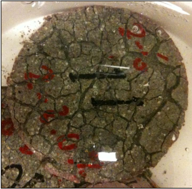
Figure 2: Damage of the mortar specimens in calcium chloride solution of 2%
