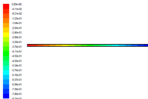
Figure 5. Contours of static pressure (Pa) along the reactor.
