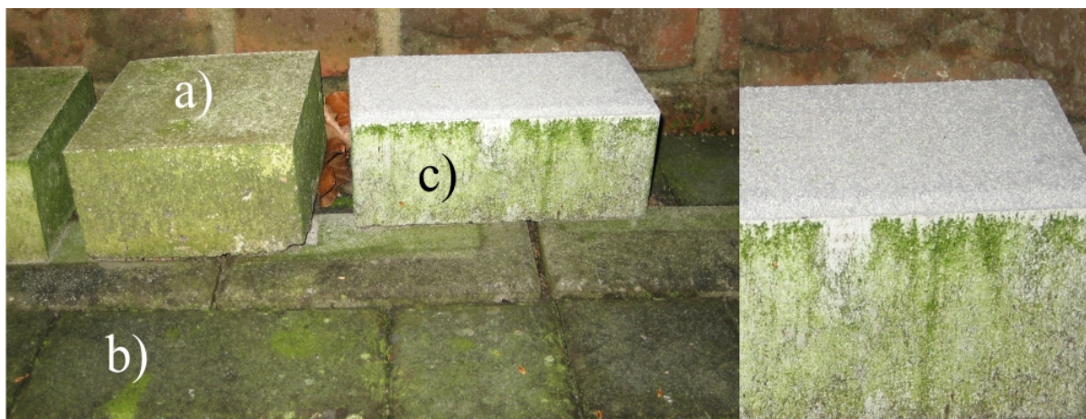
Figure 7: Staining of concrete paving blocks due to algae formation: untreated sample (a); paving of untreated paving blocks (b); paving block containing TiO 2 in the functional top layer (c)
