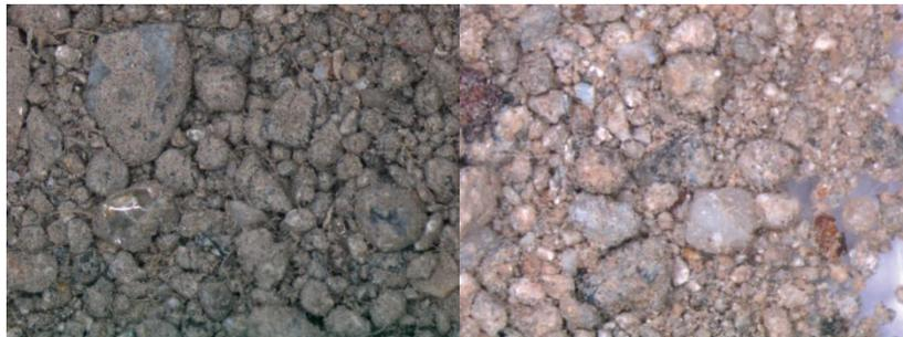
Figure 1. Bottom ash particles before (left) and after (right) 550 °C treatment (Optical microscopy)
