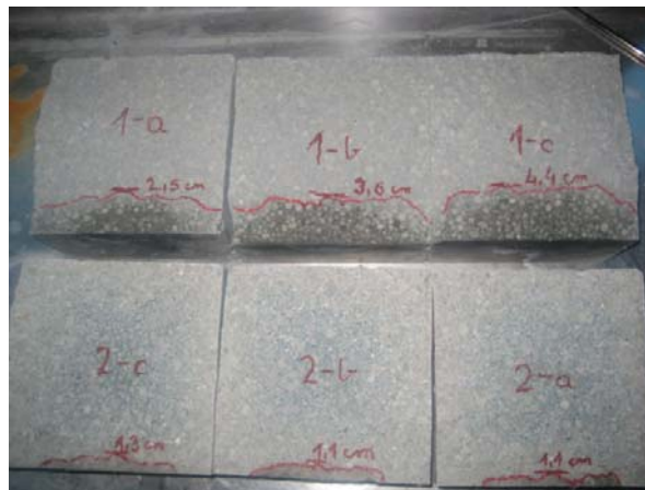
Fig. 3: The split surfaces of the LWAC after the water pressure permeability test; water ingress from the side of the bottom surface.
