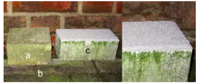
2 Staining of concrete paving blocks due to algae growth: untreated sample (a); paving of untreated paving blocks (b); paving block containing \text{TiO}_2 in the functional top layer (c)
