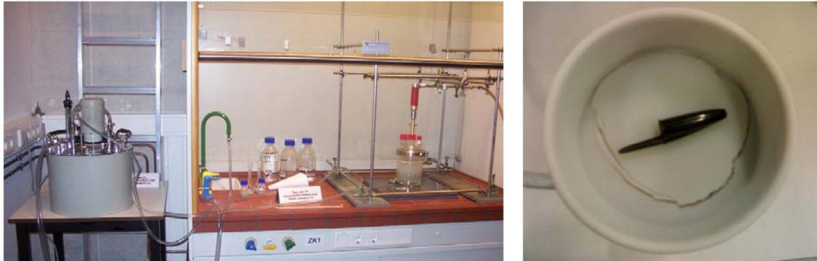
Figure 4. A) Lab scale setup for the production of olivine silica. Figure 4.B) Nano-silica produced in a stirred reactor at 70 °C and with a 3M sulphuric acid.
