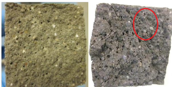
Figure 6. The fracture surface of mortars (reference and M5T)
