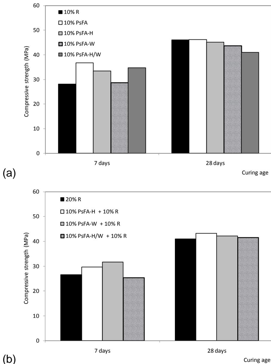
**Figure 1:** The compressive strength of PsFA-containing mortars after 7 and 28 days of curing; cement replacement of (a) 10% and (b) 20% by mass
