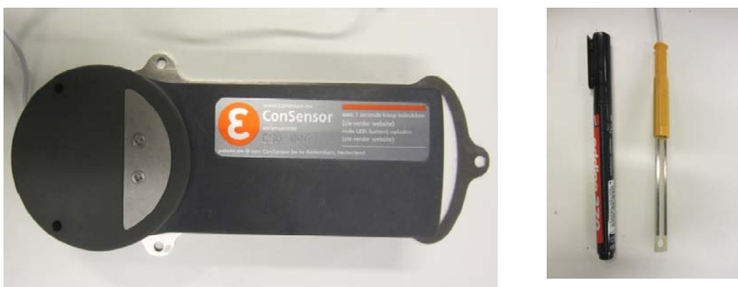
Fig. 1: Data logger (left-hand side) and conductivity sensor (right-hand side)
