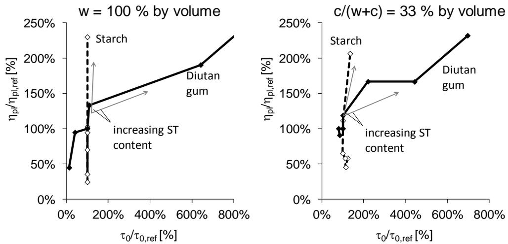
**Fig. 2:** The influence of the dosages of starch and diutan gum on  $\tau_0$  and  $\eta_{pl}$  when incorporated into water and into a water-cement suspension.
