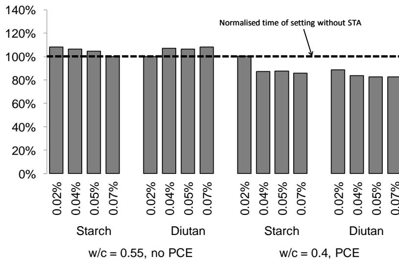
**Fig. 3:** Influence of the dosage of starch and Diutan gum on the setting without and in presence of PCE.
