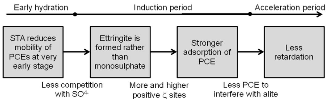
**Fig. 4:** Assumed mechanism of interaction of STA with PCE.
