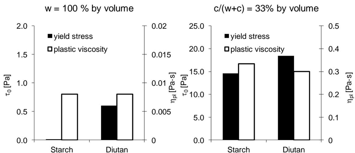
**Fig. 1:** Influence of starch and diutan gum on rheological parameters in water and water-cement systems.
